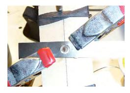
The small nickel silver piece has been given a drill-hole (between two wooden boards) sized a bit smaller than the wheel diameter. Pressed onto the soldered wheel with two clamps you lead away the heat produced while soldering the axle.
