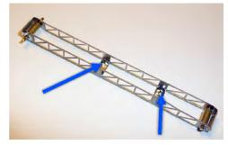
After insertion of the roller axles and the rolls the body will be soldered on the remaining open edges.
