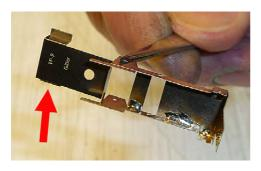
At this point it is important NOT to fold the motor housing finally but to let it in the condition shown above (red arrow). Before folding finally the steer will be mounted. After bending the motor body it will hide the screw that connects chassis and steer.
