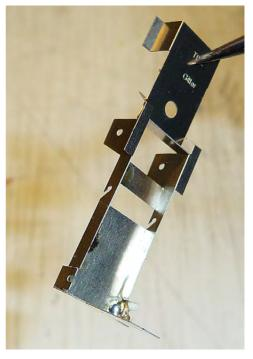
As decribed initially, the edges are pre-etched along the way they should be folded. This simplifies the way to bend but also means that the material is just half as thick on such an edge.
