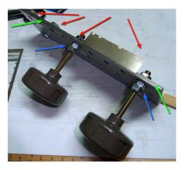
This tool uses 2 perforated plates (timber connectors) from the Do-It-Yourself-center sized  $200\times60\times2$  mm. Both plates are connected with two screws and nuts on one of the long sides of the plates. Please watch that the two plates diverge a bit — into this gap we will put the edge for bending .
