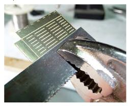
Now you bend the metal along the pre-etched edge with an appropriate piece of hardwood:
